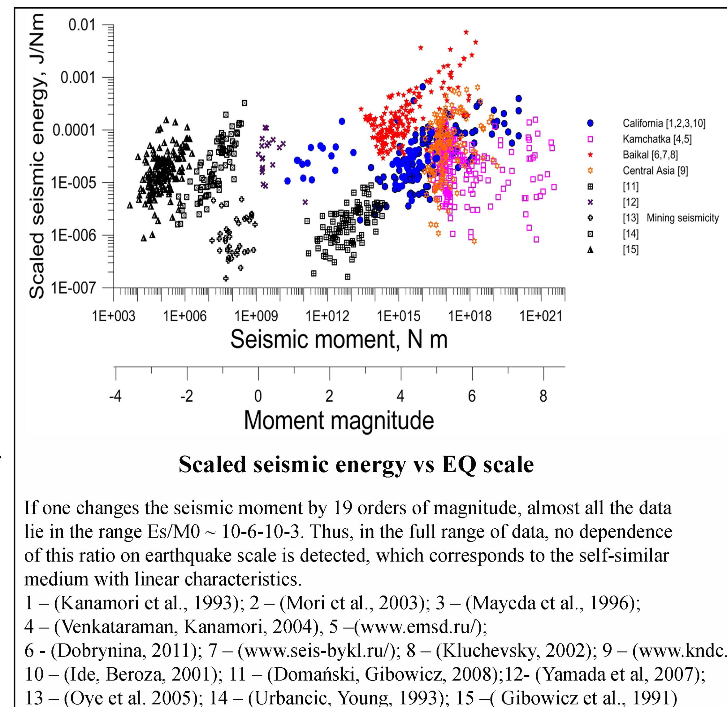
If one changes the seismic moment by 19 orders of magnitude, almost all the data lie in the range  $E_s/M_0 \sim 10^{-6}-10^{-3}$ . Thus, in the full range of data, no dependence of this ratio on earthquake scale is detected, which corresponds to the self-similar medium with linear characteristics.
