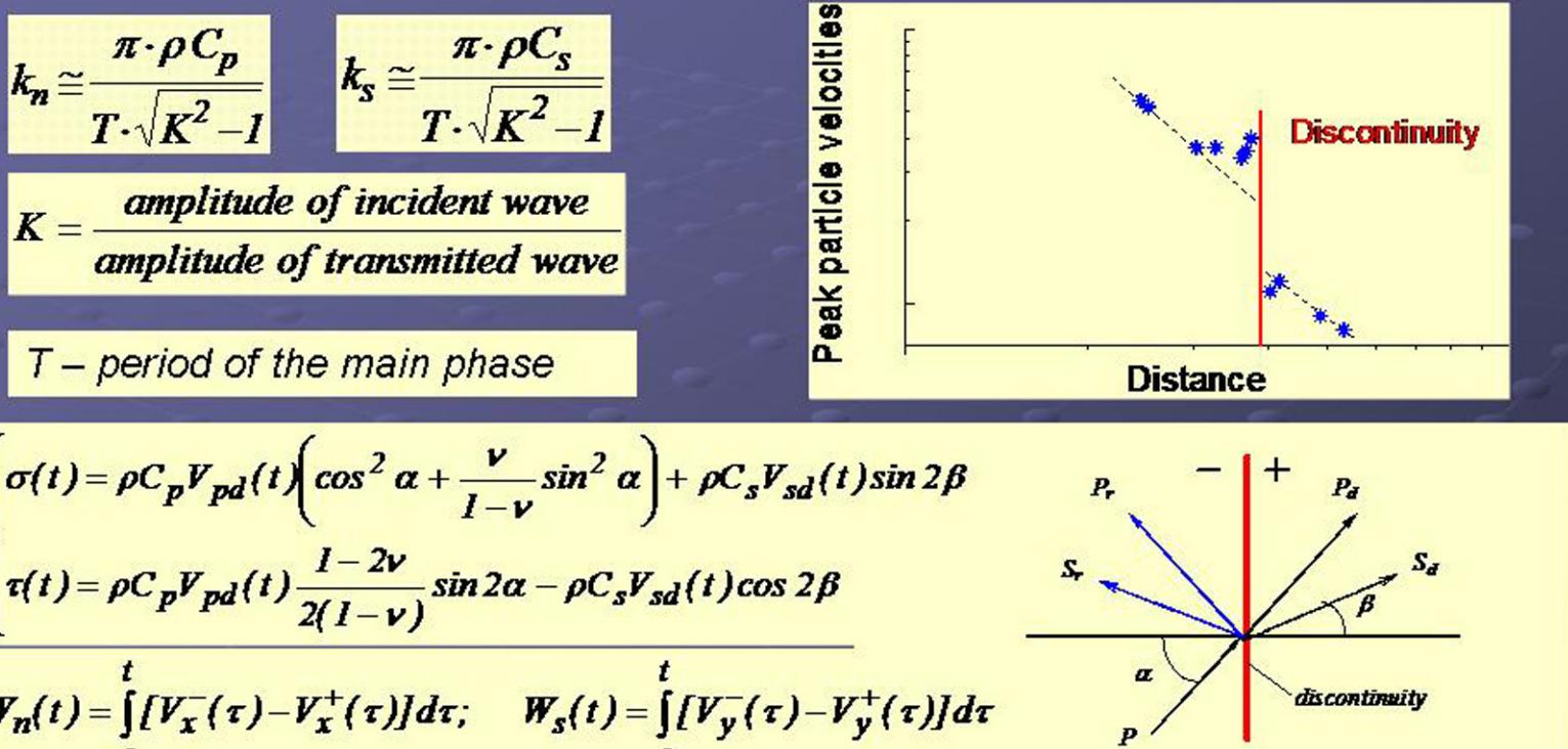
The measurements of the amplitude and time parameters of seismic waves nearly discontinuity give possibility to estimate normal and shear stiffness of the fault or fracture and even to construct stress-strain relation.
