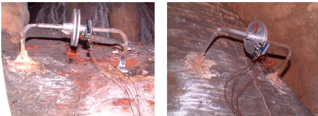
Figure 2 Photographs of extensometers P21 and P22
