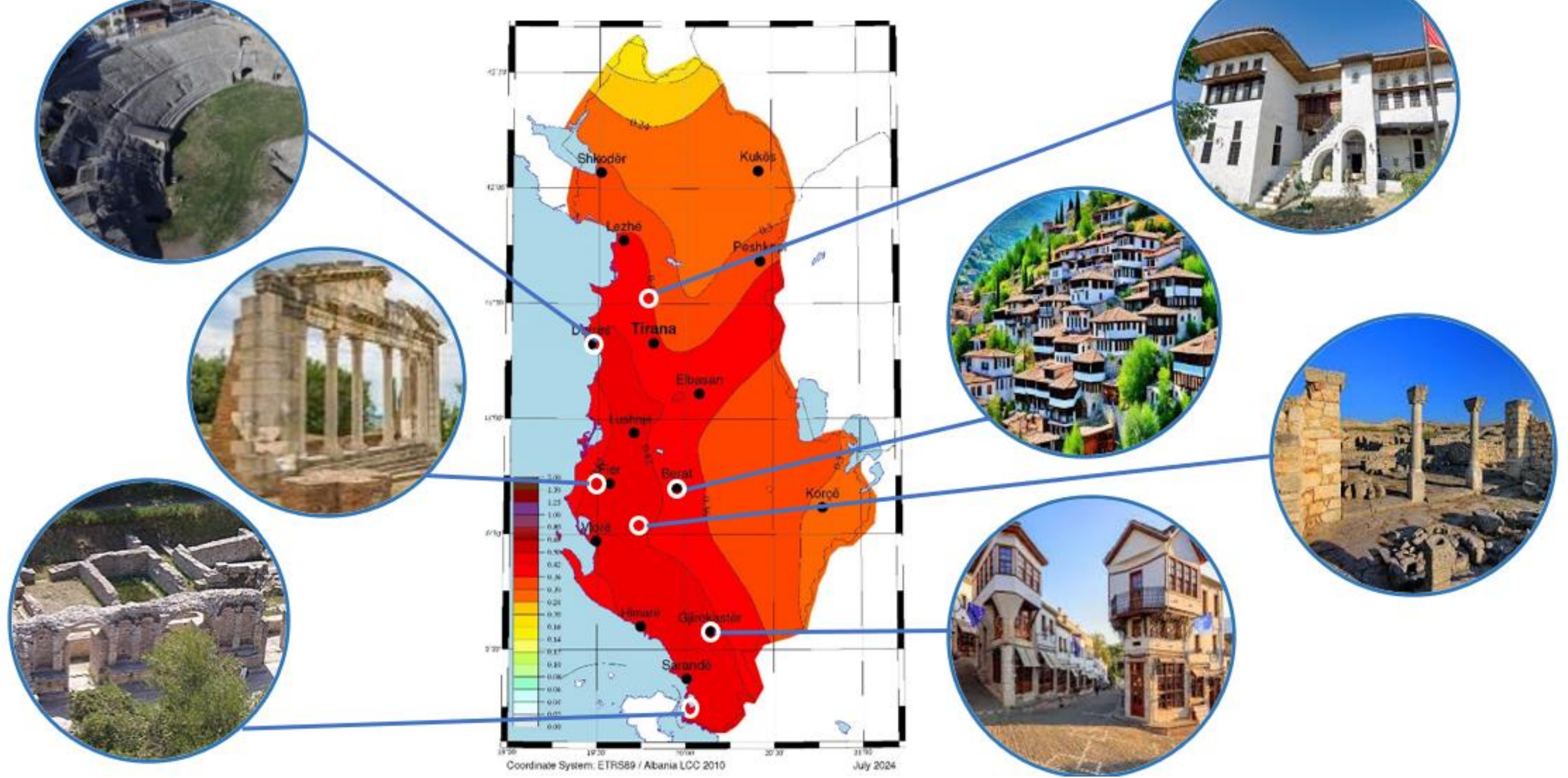
Probabilistic Seismic Hazard Map for Albania ( V_{s,30} \geq 800 m/s), PGA (10% probability of exceedance in 50 years)
