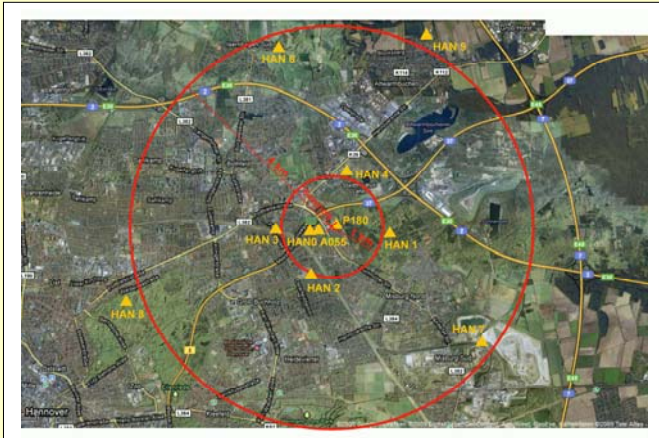
Fig. 2: Configuration of the seismic monitoring system at the GeneSys-borehole location (source of the background: Google Maps). The monitoring system consists of two circles centered at the borehole. The inner circle with 4 stations has a radius of approximately 1 km and is equipped with 4.5 Hz geophones in 100 m deep boreholes. The outer circle with radius of approximately 4 km is build up by 4 stations which are installed at the surface and equipped with 1 Hz Lennartz seismometers. Additionally, two borehole seismometers (depth 100 m and 180 m) and one broadband seismometer are maintained in direct vicinity of the borehole.
