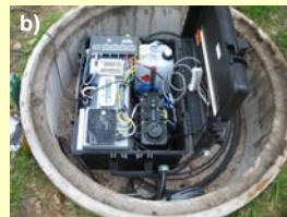
Fig. 3: a) Installation of station HAN1 b) Vault containing digitizer, battery and fuel cell c) Near real-time seismograms of station HAN0 available at the BGR internet site for the last 24 hours (update every 10 minutes). Current example covers the time span of 8 th to 9 th November 2010.
