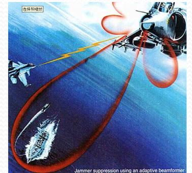
Jammer suppression using an adaptive beamformer
