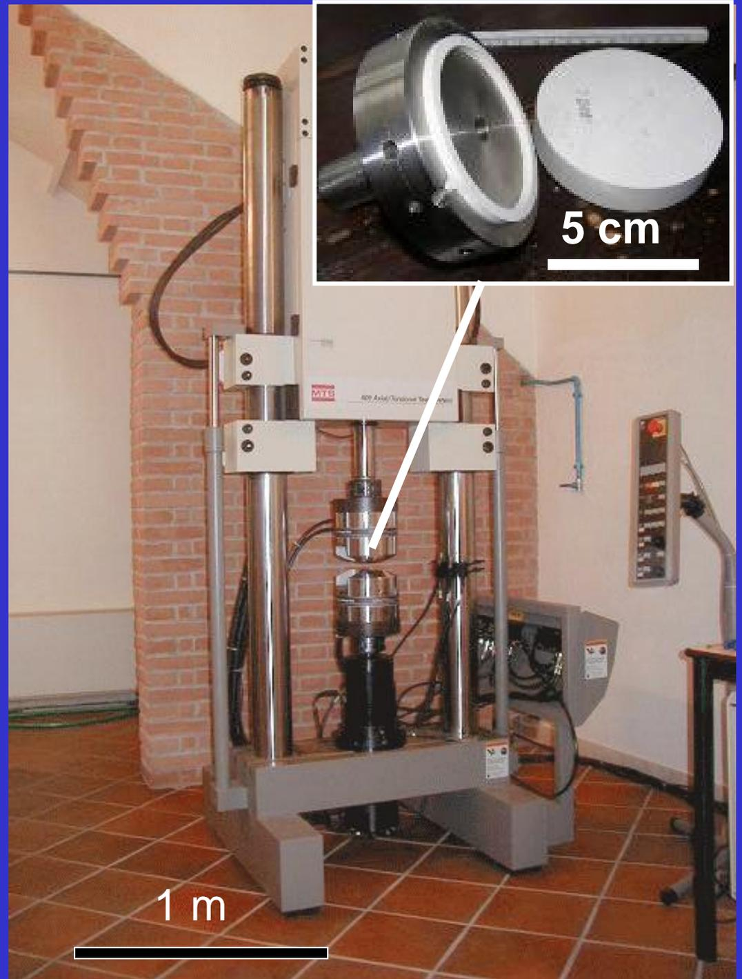
and **rotary shears** (HV-1 designed by Shimamoto, 1990)
