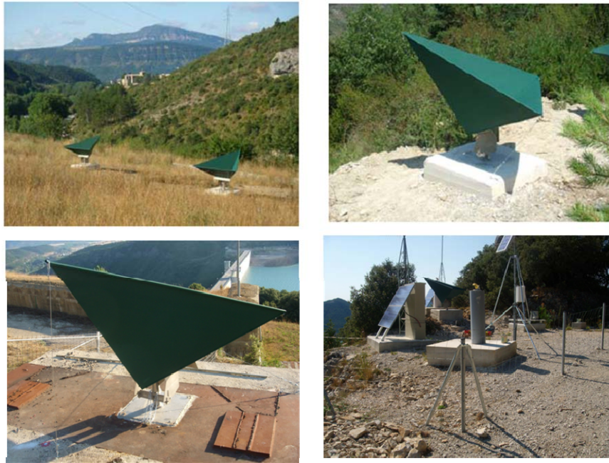
Figure 5. Some examples of corner reflectors installed in Itoiz reservoir area.
