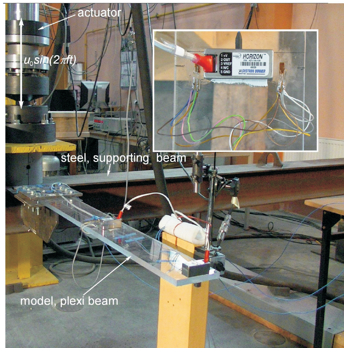
Fig. 5 Illustration of the experimental set-up to measure rotations and strains
