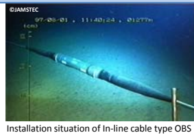
Installation situation of In-line cable type OBS
