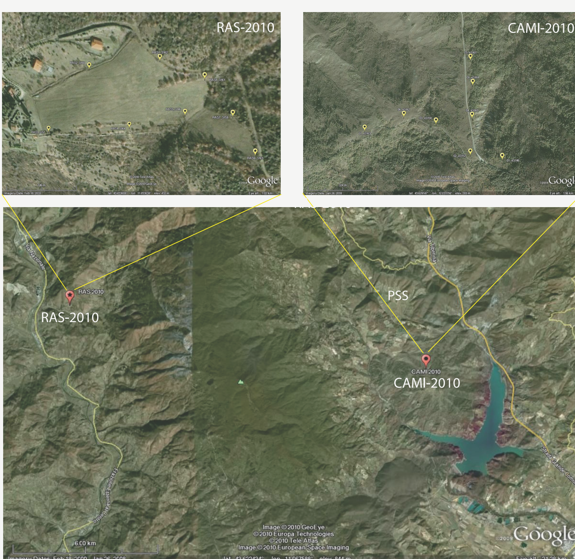
Fig. 7: Short aperture arrays installed in the study area during 2010. The RAS-2010 array was located near the epicentre of the tornillo-like events (GE in Figure 2). The CAMI-2010 array installed between near the mofettes (Figure 9), at half distance between the Montedoglio Barrier Lake and the PSS borehole. Both arrays are composed of 8 stations, equipped with Earth Data Loggers and Gural CMG-3 ESP seismometers.
