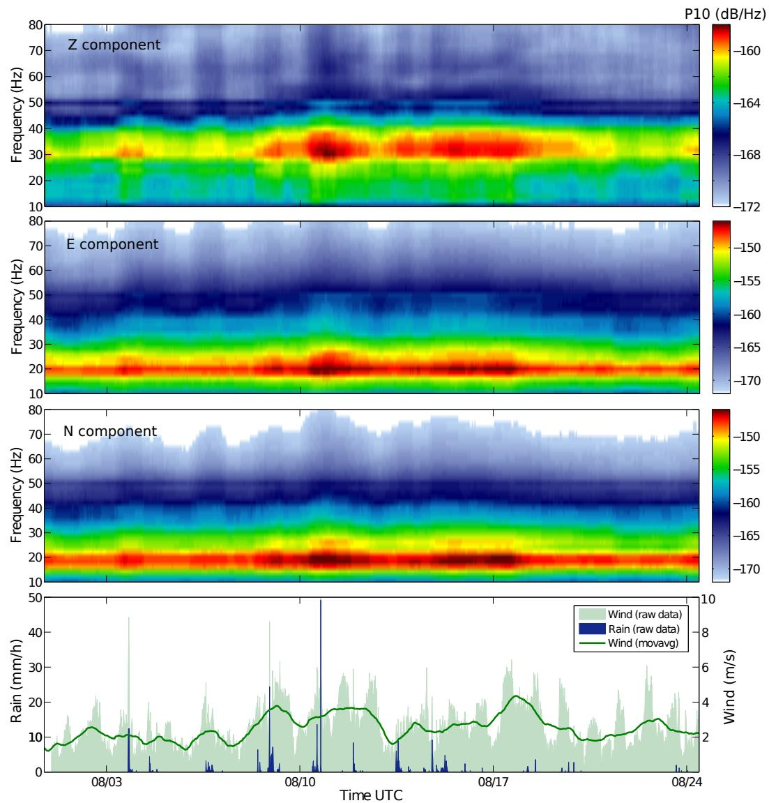
**Figure S4:** P10 for the vertical and horizontal components at S1, and wind/rain data recorded 4 km away from the area of investigation.
