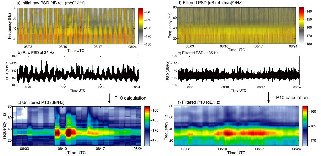
**Figure S2:** Seismic processing: **a)** Initial raw PSD map, **b)** example of raw PSD for  $f=35$  Hz, **c)** P10 extracted from a), **d)** PSD map with filtered diurnal cycles, **e)** example of filtered PSD for  $f=35$  Hz, **f)** P10 extracted from d), which corresponds to the final seismic attribute used in this study. The red line in b) and e) corresponds to the mean PSD over the entire time period.
