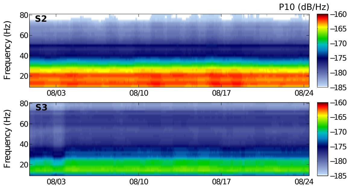
**Figure S3:** P10 for the vertical component at S2 and S3 during the August flood event, showing that no river-related signals are recorded at the two seismometers further from the stream.
