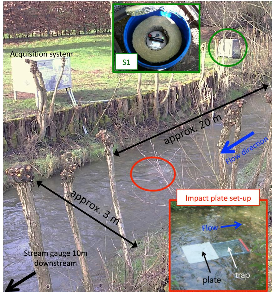
**Figure S1:** Overall equipment installed close to the stream gauge.
